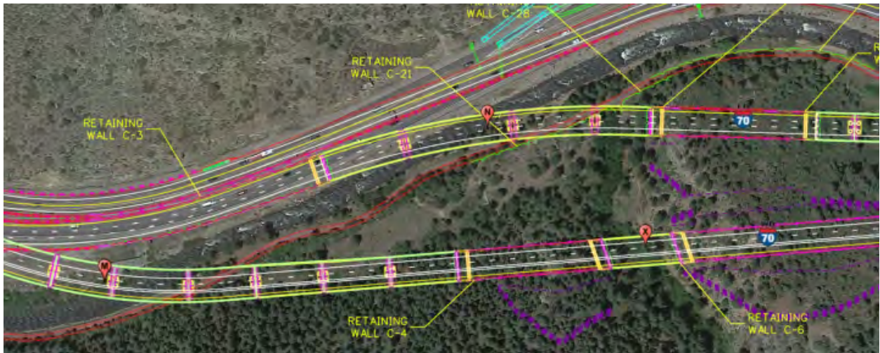
The red line above marks the trail in the fill area. The Team is looking at keeping the existing tree break next to the trail in place, in addition to revegetating the fill slope.
